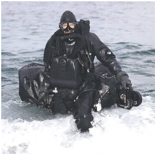
Closed Circuit Breathing Apparatus, Model LAR VI.1
